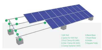
MRac Double-row Tripod Base-beam-free RMIV is derived from RM II to meet different roof projects demands. Solar modules can be arranged with single or double rows of landscape or portrait orientation. Quick installation and stable structure are assured by the modular Patented design.
