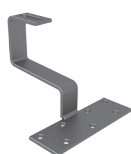
Art. 007 Pantile Roof Hook Plate: 150x50x5, (7x)Hole: Ø9mm Bar: 30x5, Long hole: 11x30 Purpose: ceramic tile, concrete tile Material: A2 1.4301 shot blasting
