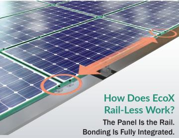
EcoX Universal Clamps and Couplings join panels together, creating a continuous structure and integrated electrical bond. This structural continuity obsoletes rails, which are no longer needed to build a strong, bonded array.
