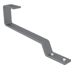
Art. 0118 Plain Tile Roof Hook Plate: 30x5, High: 265mm, Long Hole 11x29 Thickness 5mm Use: Plain Tile Material: A2 1.4301 stainless steel
