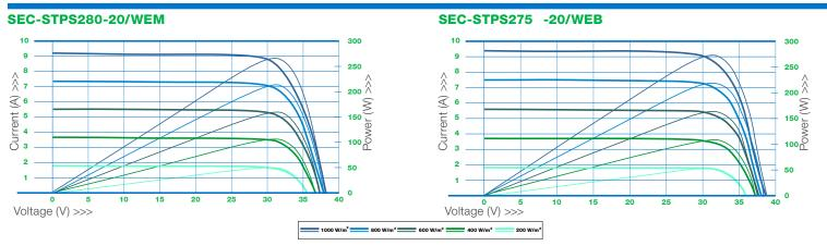
Excellent performance under weak light conditions: at an irradiation intensity of 200 W/m² (AM 1.5, 25 °C), 96.5% or higher of the STC efficiency (1000 W/m²) is achieved.
