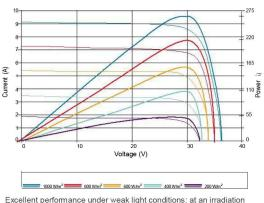
intensity of 200 W/m $^2$  (AM 1.5, 25 °C), **96.5%** or higher of the STC efficiency (1000 W/m $^2$ ) is achieved
