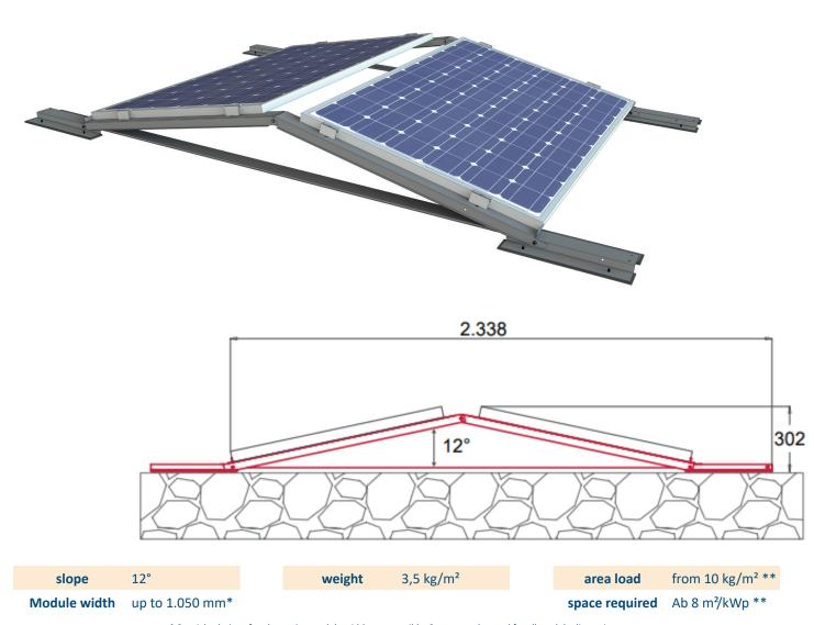
\* Special solutions for alternative module widths are possible. System can be used for all module dimensions.
