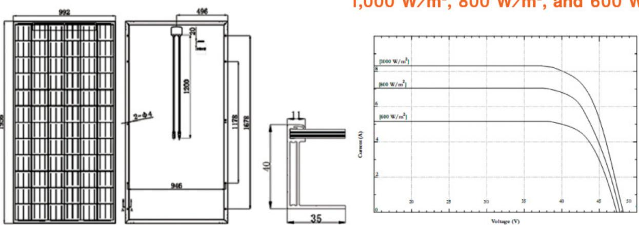
These data represent the performance of typical modules as measured at their out put terminals, and do not include the effect of such additional equipment as diodes or cables. The data are based on measurements made in accordance with ASTME1036-85 corrected to SRC (Standard Reporting Conditions, also known as STC or Standard Test Conditions), which are:
