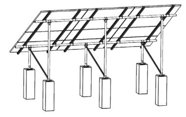
Technical Information: Install site: Open ground Tilt Angle: 10~60deg System Height: <2.5m Max Wind Speed: <60m/s Snow Load: <1.4KN/m<sup>2</sup> Standard: AS/NZS 1170 and other international Standard Material: Aluminum alloy Al6005-T5& Stainless steel 304 & Hot galvanized steel Anticorrosive: Anodized & Hot galvanized Color: Natural or Optional Warranty: 10 years warranty and up twenty years service life
