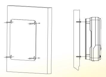
Figure 2-2 Fix the solar charge controller
