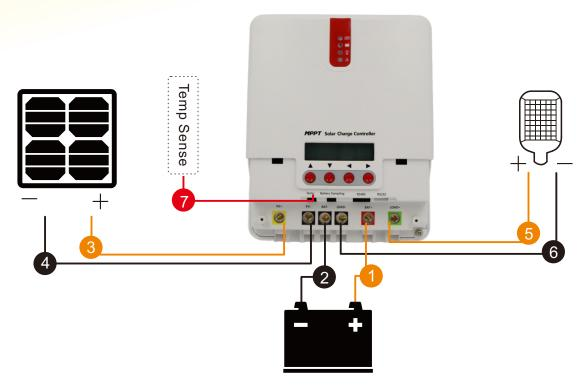
Figure 2-3 Wiring
