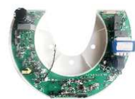
MPPT water heating controller
