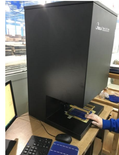
Cell efficiency test machine
