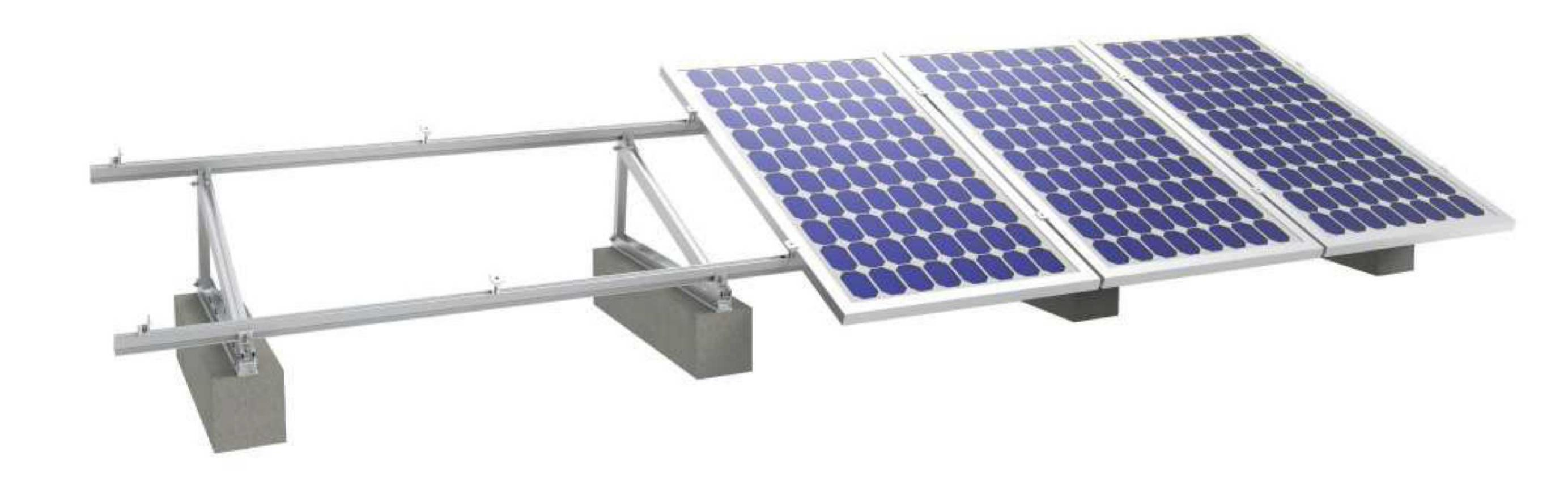
AS Solar Tripod Concrete Roof Solar Mounting System is designed for solar installation on concrete flat roof. Tilt angle can be customized between 5° and 45° based on each project. With concrete base as foundation, this system also applies for ground-mount solar installation.
