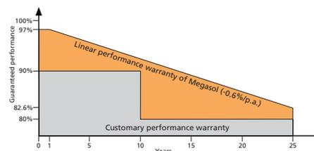
Relative efficiency level in relation to the minimal output (%). At least 97% of the minimum output during the first year. Afterwards, max. 0.6% degradation per annum. At least 91.6% of the minimum output after 10 years. At least 82.6% of the minimum output after 25 years. All data within the measuring tolerances. Warranties according to the respective latest Megasol Warranty Conditions which can be found on [www.megasol.ch/warranty](http://www.megasol.ch/warranty).
