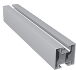
Art. 0111 Mounting Rail 40 type I Measurements: 40x40 Length: 6200mm, 3100mm, 2070mm Joining screws: top M8, bottom M10 Material: AL6060T6
