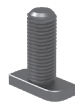
Art. 0129 Hammerhead screws 28/15 Measurements: M8 16 +70 M10 16+100 Use: Mounting Rail Art. 0110 Material: A2 1.4301 stainless steel
