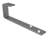
Art. 015 Slate Tile Roof Hook Plate: 30x5, Length 235mm (2x)Hole: Ø9mm, Long Hole: 11x29 Thickness 5mm Use: Slate Tile Material: A2 1.4301 stainless steel
