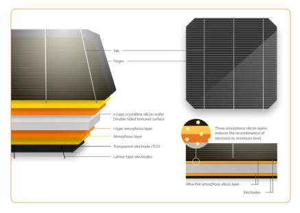
Panasonic HIT® KURO is our all-black module which features a high module efficiency of 19.7%, an industry leading temperature coefficient of -0.258% /°C and a sleek design.
