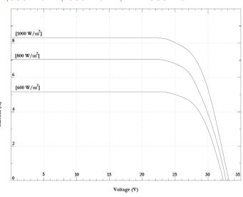
These data represent the performance of typical modules as measured at their out put terminals, and do not include the effect of such additional equipment as diodes or cables. The data are based on measurements made in accordance with ASTME1036-85 corrected to SRC (Standard Reporting Conditions, also known as STC or Standard Test Conditions), which are:
