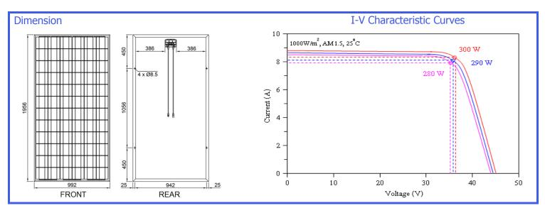
Electrical specification are based on measurements performed at standard test conditions (STC) of 1000 W/m<sup>2</sup> irradiance, air mass 1.5 and cell temperature of 25°C after long-term stabilization. Performance may vary up to 10% from rated power due to temperature operation, spectrum and related effects.
