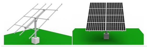
Empery Pole Mounting System is the perfect solution when maximum flexibility is required in the installation. A single, free standing support pole can accommodate 4, 6, 8 or 10 panels. Any number of poles can be installed to grow the system. Poles can be rotated to the optimum orientation, and the system of panels on each pole can be turned to any one of five angles: 10, 20, 30, 40 or 50 degrees to maximise power generation.
