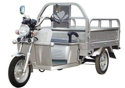
Application: Electric Van Voltage: 48V Capacity: 200AH Cell: 3.2V 200AH prismatic cell Pack: 16S1P
