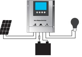
Please observe that the automatic adjustment to 12V/24V systems does not function properly, if this sequence order is not followed. An improper sequence order can damage the battery!
