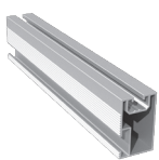
Art. 0109 Mounting Rail Measurements: 31x50 Length: 6200mm, 3100mm, 2070mm Joining screws top: M8 side: M8/M10/M12 Material: AL 6060T6
