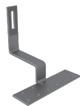
Art. 093 Pantile Roof Hook Standard Plate: 180x50x4, (12x)Hole: Ø7mm Bar: 30x5, long Hole: 9x47 Use: pantile roof Material: A2 1.4301 stainless steel, shot blasting
