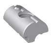
Art. 080 T-slot nuts, self aligning with spring ball M8 Used with hexagon socket cap screw Art. 0132 Use: for Mounting Rails Art. 0109, Art. 0110, Art. 062, Art. 0111, Art. 0112 Material: AL 6060T6
