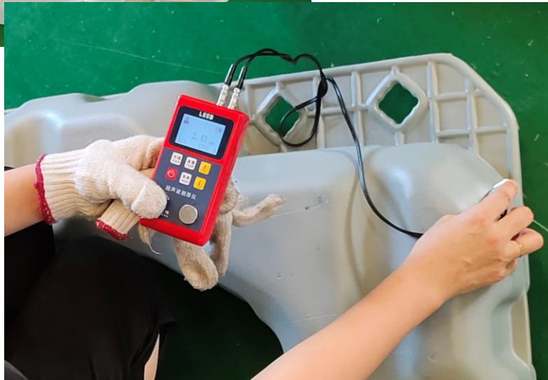
Inspection for wall thickness of floater body
