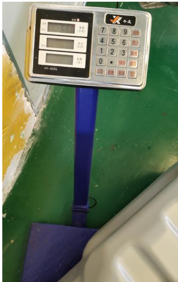
Floater weight inspection
