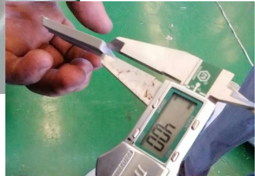
Inspection for the wall thickness of joint line
