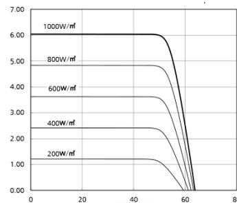
Reference data for model VBHN300SJ46 (Cell temperature: 25°C)
