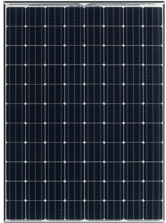
Our slim Panasonic HIT<sup>®</sup> N300 features a high module efficiency of 19.5%, an industry leading temperature coefficient of  $-0.258\% / ^\circ\text{C}$  and a sleek design. Powerful and efficient, designed to get the most out of your roof!
