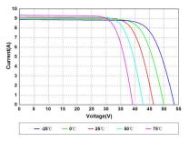
Current-Voltage Curves at Different Temperatures
