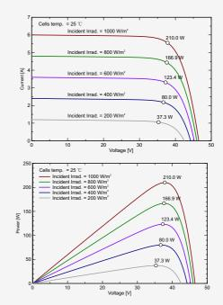
STC: Irradiance 1000W/m<sup>2</sup>,Module temperature 25°C,AM1.5 spectrum.
