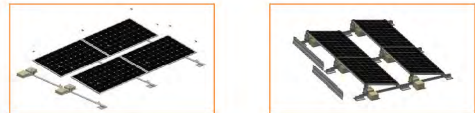
2. Using end clamp and mid clamp fixed solar module on aluminum rails
