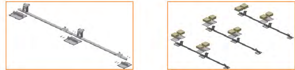
1. Rely on request of drawing. fixed clamp on relevant place of tin roof
