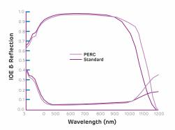
PERC technology enables better light capturing abilities at longer wavelength, weak and diffused light and in cloudy conditions.
