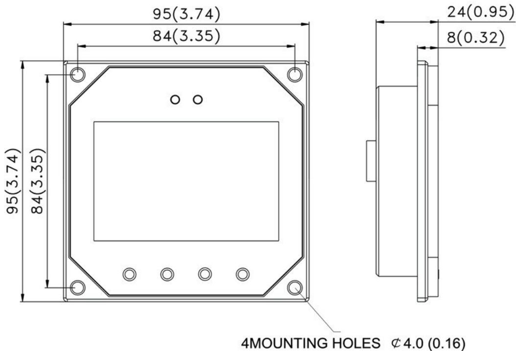
**NOTE:** Dimensions are in millimeters (inches)
