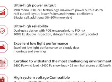
High system voltage Compatible Maximum 1500V DC system voltage saves total system cost
