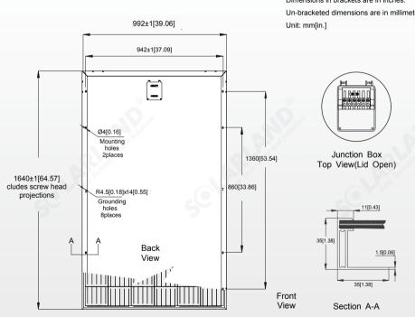
Dimensions in brackets are in inches Un-bracketed dimensions are in millimeters.
