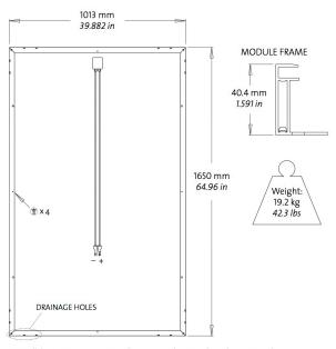
NOTE: All dimensions are accurate within ±1.5mm tolerance unless otherwise stated. Product dimensions in imperial inches (conversion of 1mm equals 0.03937in,1kg equals 2.2lbs) are provided for information purposes only.
