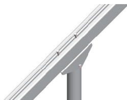
② Connection of hinge base and column
