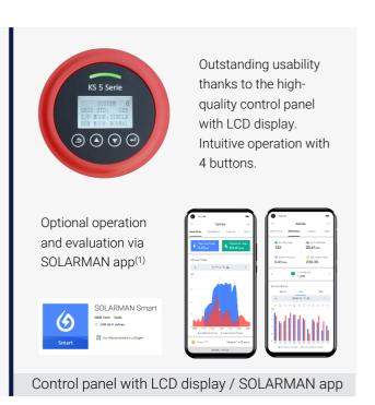
(1) To operate the SOLARMAN app, the mobile device must be connected to the solar inverter via WiFi (optional WiFi plug).
