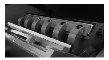
The slanted rotating knives work in conjunction with stationary opposed slanted bed knives mounted in the granulator housing.
