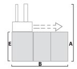
Machine weight total: 803/618 kg bale chamber only: 196/196 kg bin chamber only: 450/265 kg press unit only: 157/157 kg
