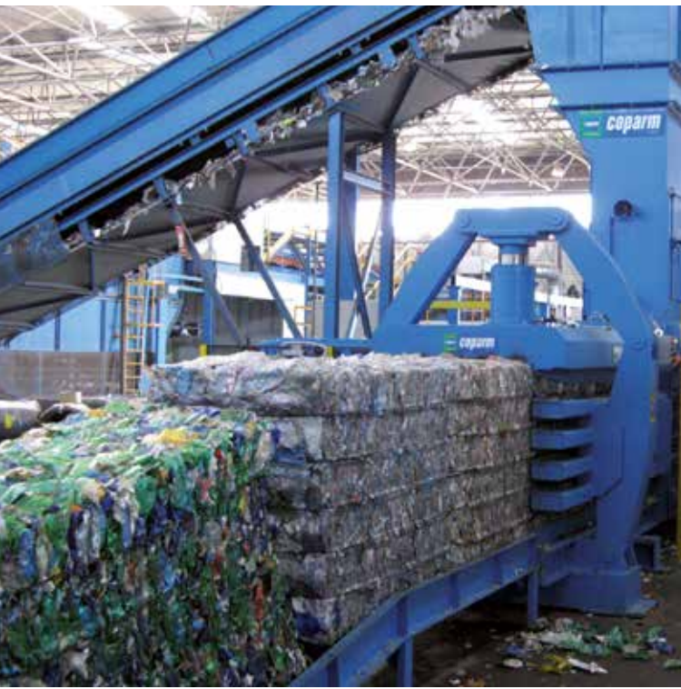
Pressa mod. PR 50 imballaggio PET - Baler mod. PR 50 PET packaging
