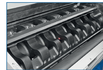
3 or 5 knives rotor with scissors-cutting configuration
