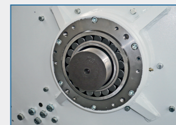
Swinging roller bearings on pressure compass mounted to the grinding chamber, supports in cast iron
