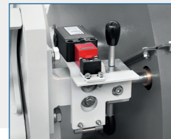
Rotor lock device for maintenance
