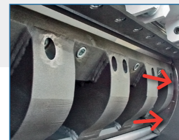
Rotary discs integral with the rotor and rings Discs fixed to the chamber (optional)
