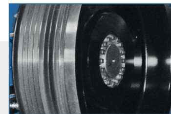
Keys for the fixing of motor pulley and flywheel Pulley and flywheel manufactured as per drawing due to high inertia
