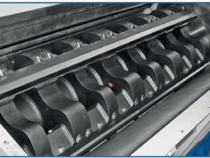
3 or 5 knives rotor with scissors-cutting configuration
