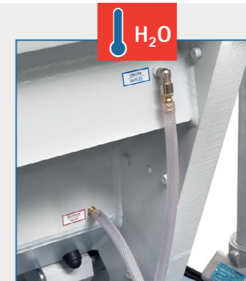
Chamber water cooling
