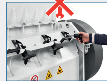
Access without tools to the main maintenance parts
