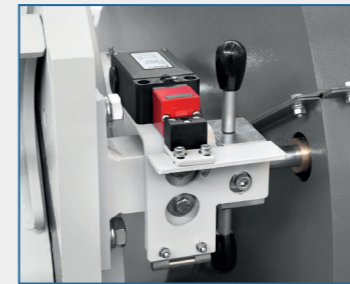
Rotor lock device for maintenance
