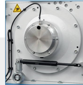
Screen-holder opening by gas cylinder
