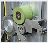
Cantilevered design of cutting and draw-in section
