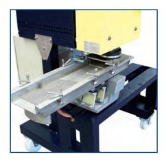
Classifier integrated into the machine frame
