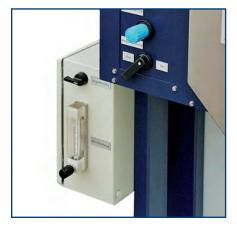
Cutting area cooling with cool-air volume throughput display
