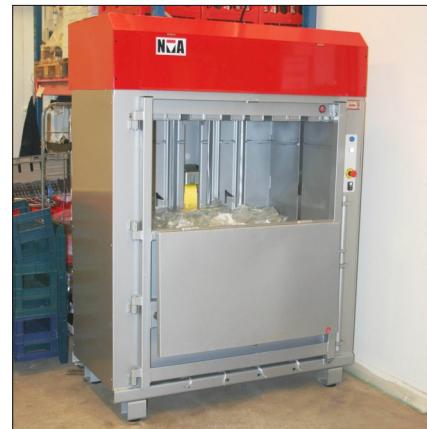
The feed door is opened 90° as standard but can be opened all the way down 180°, adjusted to your needs.
