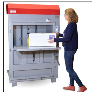
Low loading height, generous feed volume. Close the feed door for automatic compaction.
