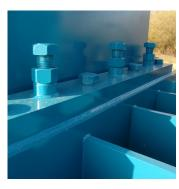
The Galaxy2R® wide model features an adjustable shear beam that enables you to adjust the shear blades from the exterior of the machine.
