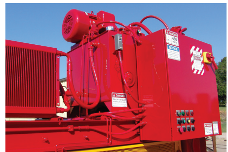
High-efficiency power unit and electrical disconnect.
