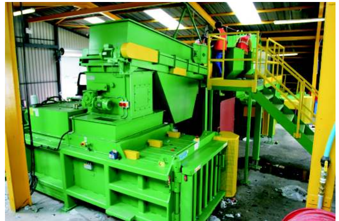
Left: ME70 with hopper and conveyor from door end. Above: side view showing easily accessible service points. Below: bale being easily handled with use of pallet truck.
