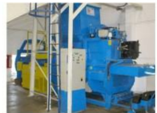
Tetrapak at Wrexham use their HB50 for baling waste plastic and off-cuts from their well-known cartons.
