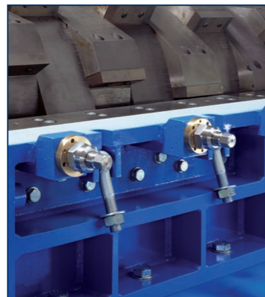
cutter clearance adjustable from outside
