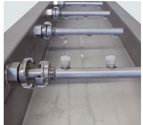
Quick-change spray tubes for simple maintenance during operation
