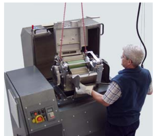
Replacing the cutting head
