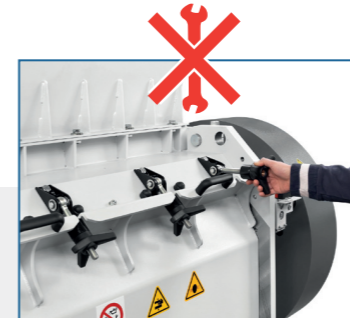
Access without tools to the main maintenance parts
