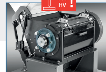
Grinding chamber in anti wear execution
