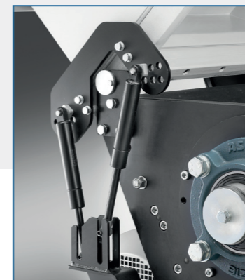
Hopper opening by gas cylinder
