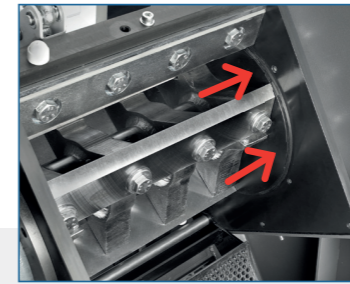
Rotary discs integral with the rotor and containment rings
